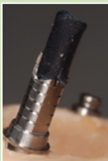
Place the Extragate titanium abutment with the short screw onto the Ot Equator attachment, making sure to place the flat surface of the titanium abutment in correspondence with the undercut created by the implant inclination. It is recommended to protect the screw hole with a wax pin.
