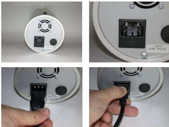
Connect the provided power cord with the socket on the rear panel of the base unit and plug it into a power outlet.
