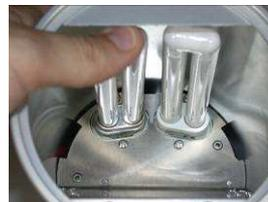
When ordering new lamps (your domestic dealer or primotec, Bad Homburg) please pay attention to the correct wave length, as there are two different lamps installed in Metalight Mini.
